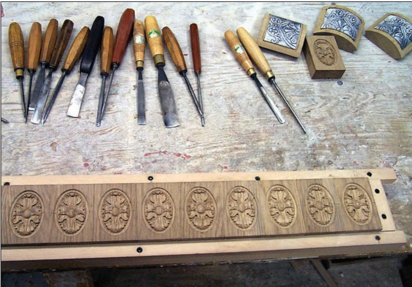
Foliolate medallions for the replica Resolute Desk being hand carved in the Eli Wilner Studio (above); An artisan in the Eli Wilner studio assembles a replica of the Resolute Desk (right)
