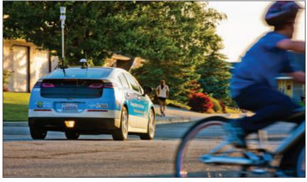
PG&E bas begun using car-mounted gas leak detection technology that is 1,000 times more sensitive than traditional equipment.
