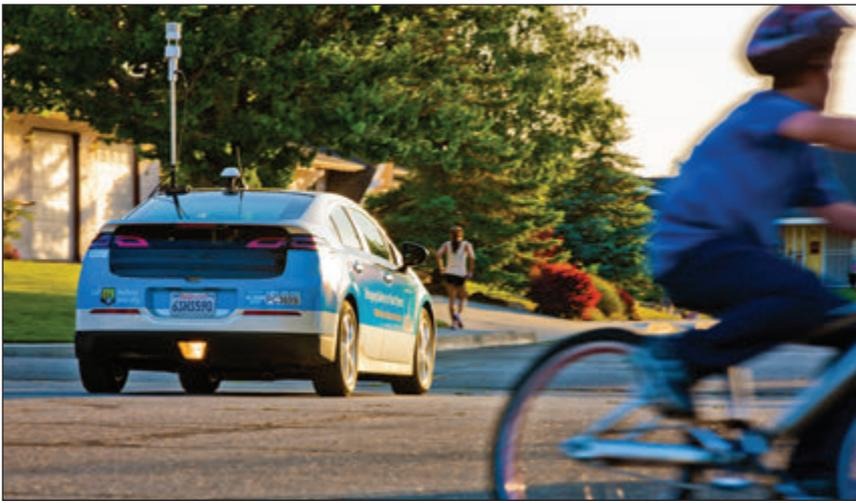
*PG&E has begun using car-mounted gas leak detection technology that is 1,000 times more sensitive than traditional equipment.*
